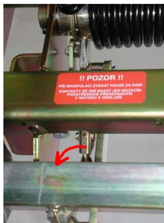
OFF position break lever (front view)
